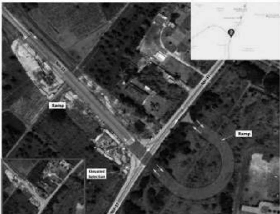
Figure 139 Intersection 2 Proposed Grade Separation
