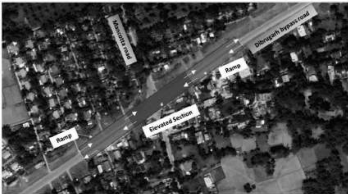
Figure 141 Proposed Grade separator on Bypass Road at Khanikar Charai
